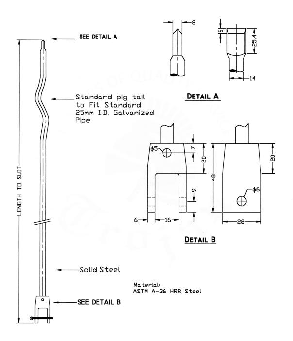
c/w RIVET ATTACHED CAST CLEVIS
